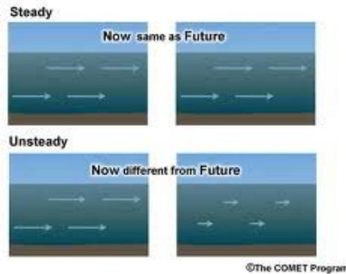
In steady flow streamlines and streaklines do not vary with time and coincide with the pathlines.
