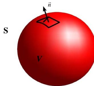
$$\text{LHS:} \quad \frac{d}{dt} \int_V \rho dV = \int_V \frac{\partial \rho}{\partial t} dV$$
