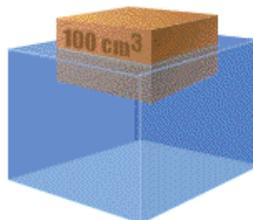
Volume of water displaced =  $60 \text{ cm}^3$
