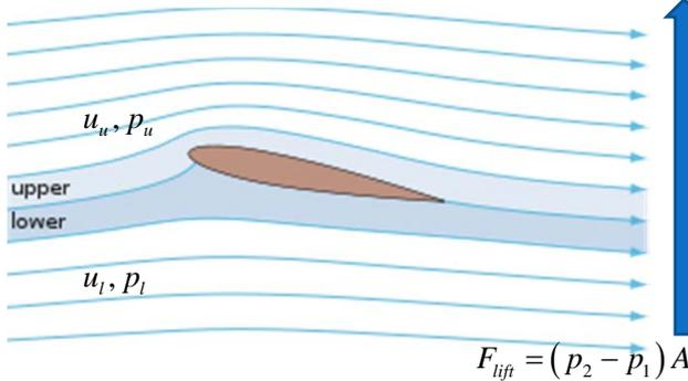
Along the wing, the flow over the upper (longer) edge of the wing has a (considerably) higher velocity  $u_u$  than below the wing,  $u_l$ .
