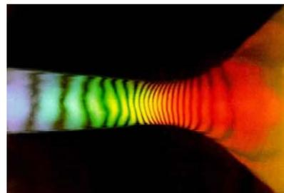
Two illustrations of the de Laval nozzle principle. The 2<sup>nd</sup> figure is a measurement of the flow speed in an experiment.
