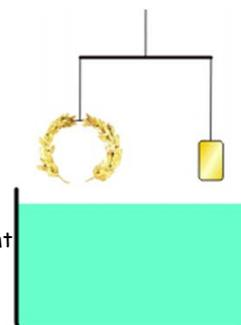
$$\text{Buoyancy} = \text{Weight of displaced fluid}$$
