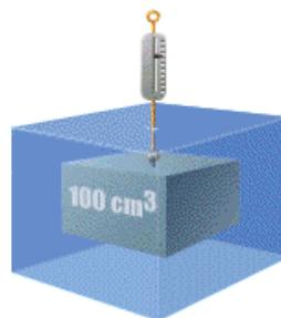
Volume of water displaced =  $100 \text{ cm}^3$
