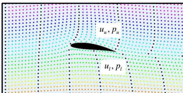
Flow around an airfoil: the dots move with the flow. Note that the velocities are much higher at the upper surface than at the lower surface. The black dots are on timelines, which split into two — an upper and lower part — at the leading edge. The part of a timeline below the airfoil does not catch up with the one above! Colors of the dots indicate streamlines.
