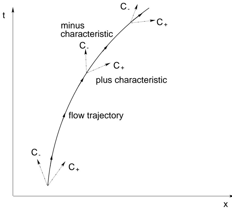
Figure 7.1: Diagram showing the space-time flow line, defined by  $dx = u dt$ , and the two characteristics  $C_+$  and  $C_-$  defined by  $dx = (u + c_s) dt$  and  $dx = (u - c_s) dt$ . From each point in the flow two characteristics originate along which  $C_+$  and  $C_-$  are constant respectively. Note that the value of  $C_{\pm}$  can be different on the different characteristics so that the characteristic variables  $C_+$  and  $C_-$  are **not** global constants!
