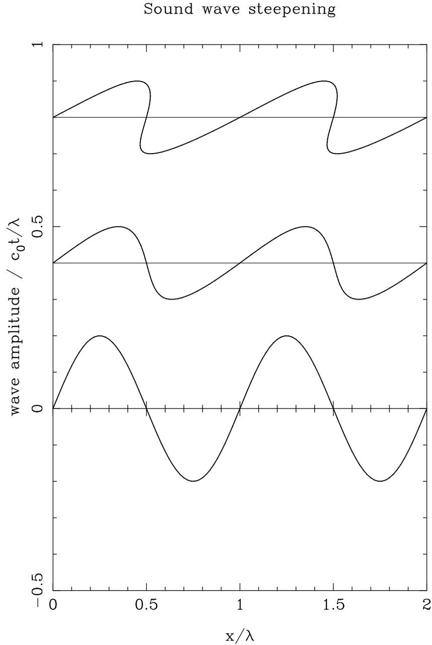
Figure 7.3: *The shape of an initially sinusoidal sound wave at  $t = 0$ ,  $c_{s0}t/\lambda = 0.4$  and  $c_{s0}t/\lambda = 0.8$ . The sound wave steepens. Before the plus-characteristics cross at  $c_{s0}t/\lambda = 0.4$  it has a saw tooth-like shape. After the crossing of the characteristics at  $c_{s0}t/\lambda = 0.8$  the shape is double-valued, and hence unphysical near the nodes at  $x/\lambda = 0.5$  and  $1.5$ . Before that, a shock will form at these nodes.*
