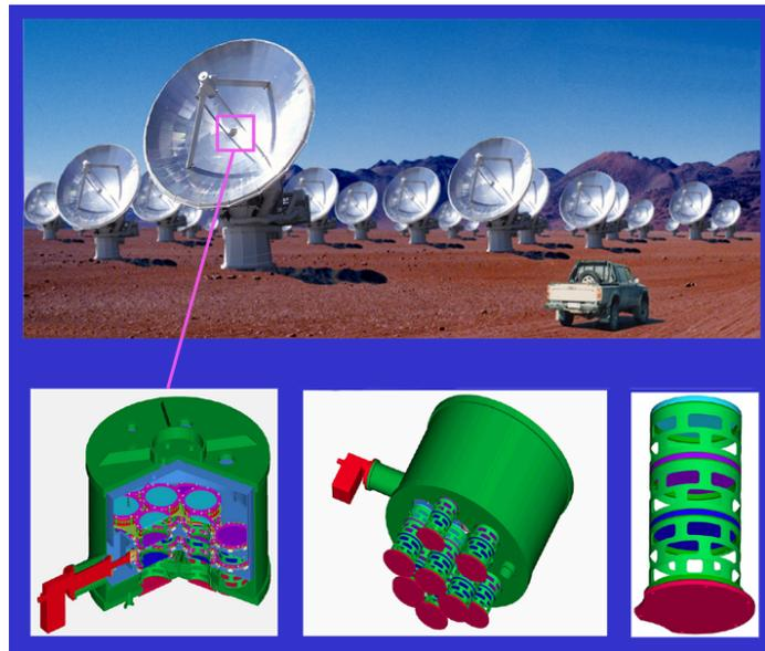
In the focal plane of each 12-meter dish, 10 cartridges with detectors for different frequency-bands will collect (sub)millimeter radiation and convert this to a signal with lower frequency, permitting electronic processing. In this way, the 64 telescopes can be made into one giant virtual telescope with .01 arc second resolution, much better than any stand alone optical or radio telescope.
