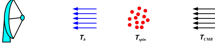
Fig. 14 A cartoon that shows that set up of the various components relevant to radiative transfer problem at hand starting from the background (CMB) radiation, going through a certain cloud with temperature T_{spin} and emerging with a temperature T_b that is measured by our telescopes
