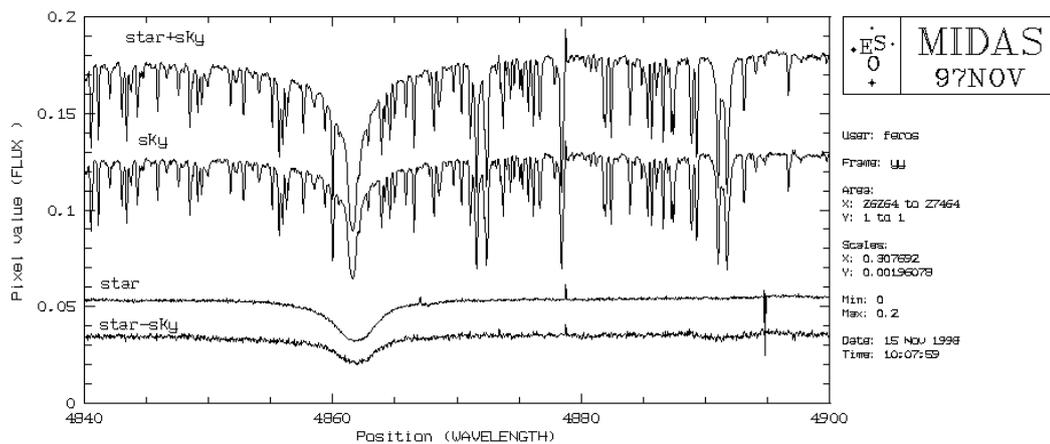
FIGURE 2.2: Example of a sky removal from a spectrum. With a star+sky and sky data given, star data can be obtained. Taken from <https://www.lsw.uni-heidelberg.de/projects/instrumentation/Feros/Installation.html>.
