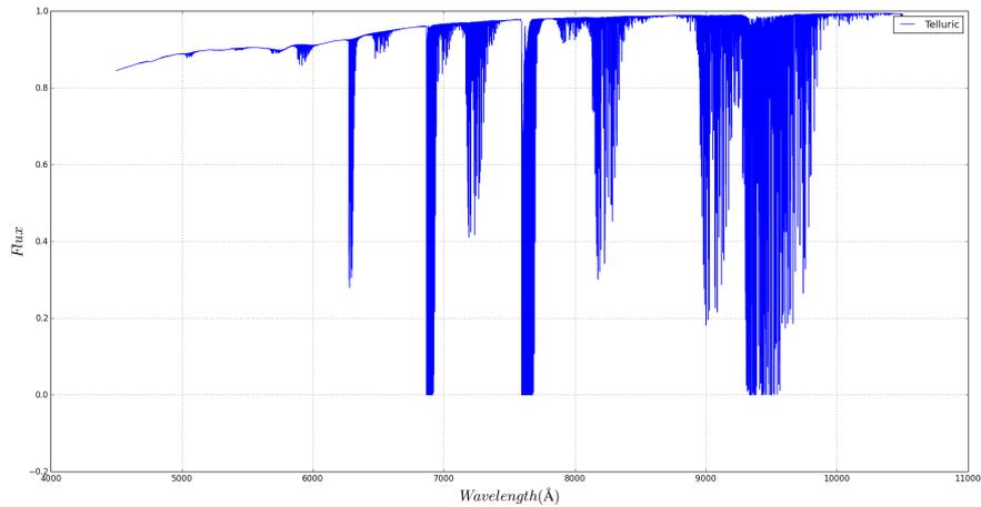
FIGURE 3.1: Normalized telluric spectrum taken from TAPAS (Bertaux, 2014) for a region 4500-10500 Å. If flux values are at 1 it means that no radiation is absorbed by the atmosphere, if flux values at 0 - all radiation is absorbed by the atmosphere in this region.
