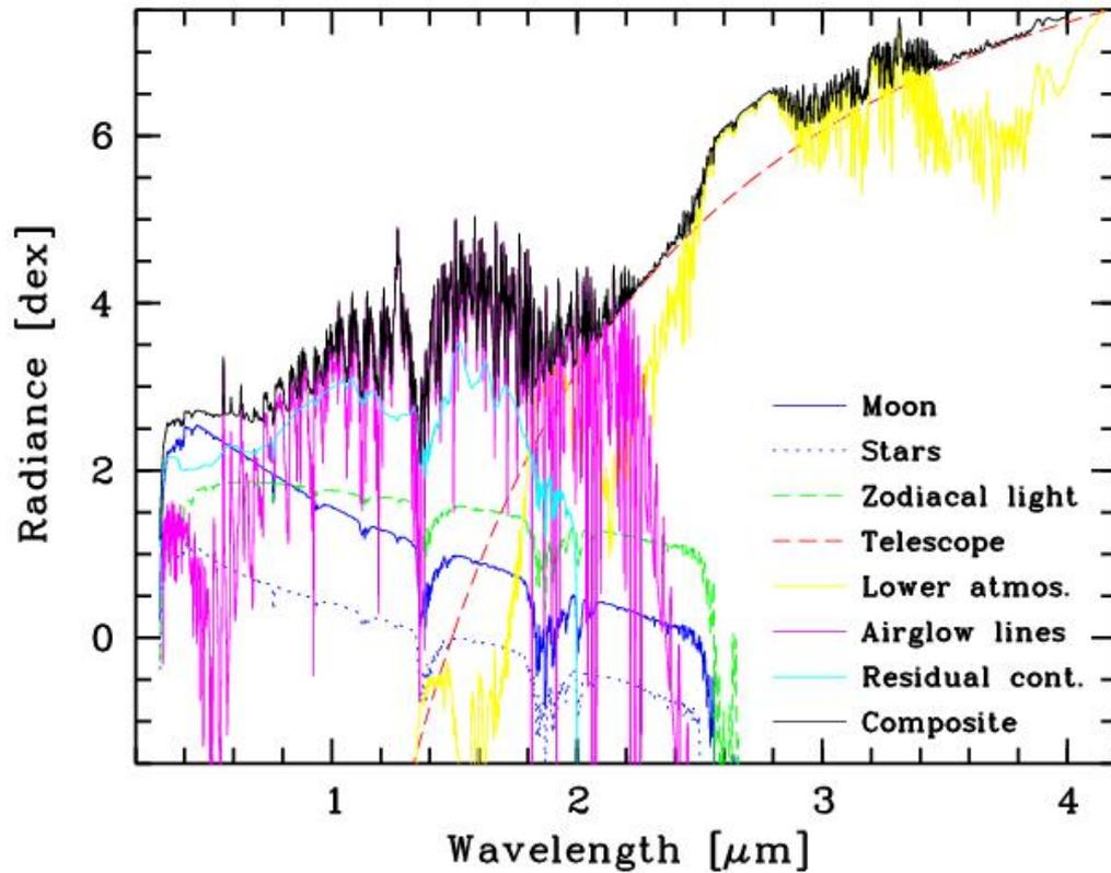
FIGURE 2.1: Components of the sky model in logarithmic radiance units for wavelengths between 0.3 and 4.2  $\mu\text{m}$ . This example, with the Moon above the horizon, shows scattered moonlight, scattered starlight, zodiacal light, thermal emission by the telescope and instrument, molecular emission of the lower atmosphere, airglow emission lines of the upper atmosphere, and airglow/residual continuum.
