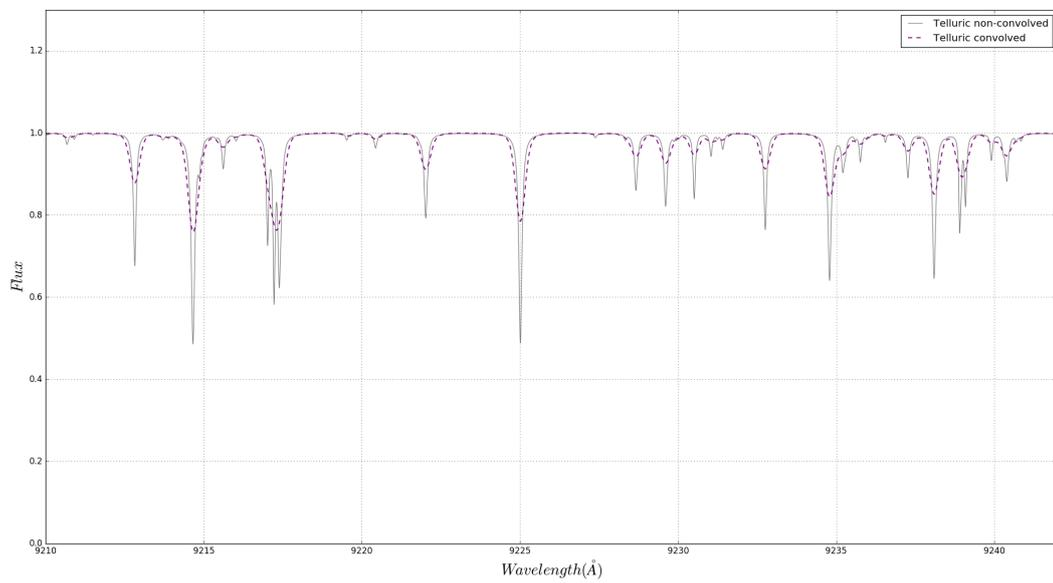
FIGURE 3.2: Telluric convolved with Gaussian ( $\sigma=70$ ) is shown as a dotted purple line. Gray line is non-convolved synthetic telluric
