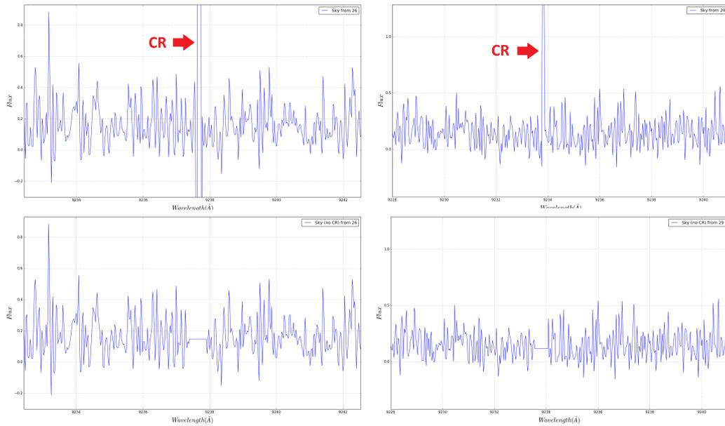
FIGURE 2.4: Two different sky spectra on the top have CR in the region between 9210 and 9242 Å. On the bottom spectra CR are removed by taking the median around them.
