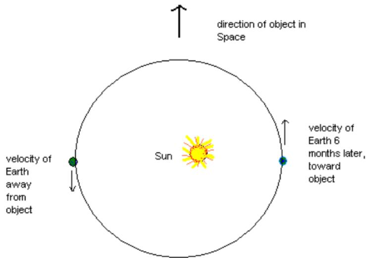
FIGURE 4.1: Earth motion around the sun that produced Doppler Shifts in the object of interest. From (Wood, 2003).
