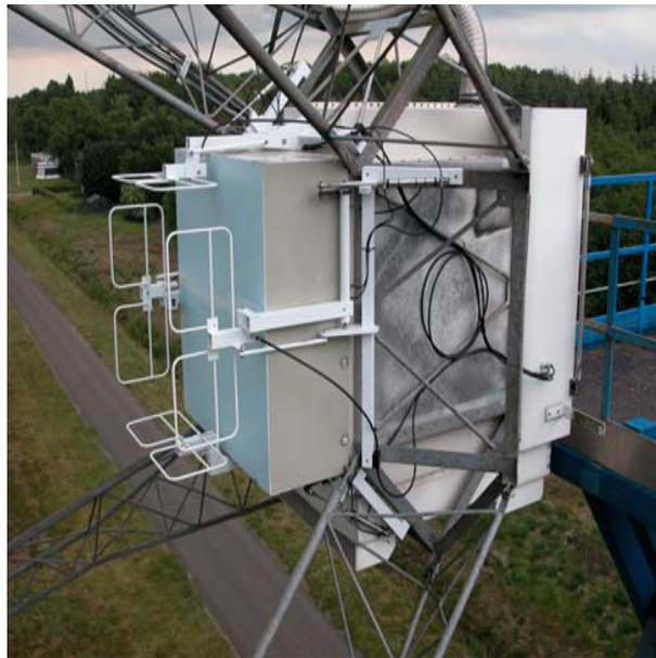
Figure 1.2: *An LFFE consists of four folded dipole antennas: two for each linear polarization. The dipoles can be moved to prevent blocking the MFFE (photo Astron).*
