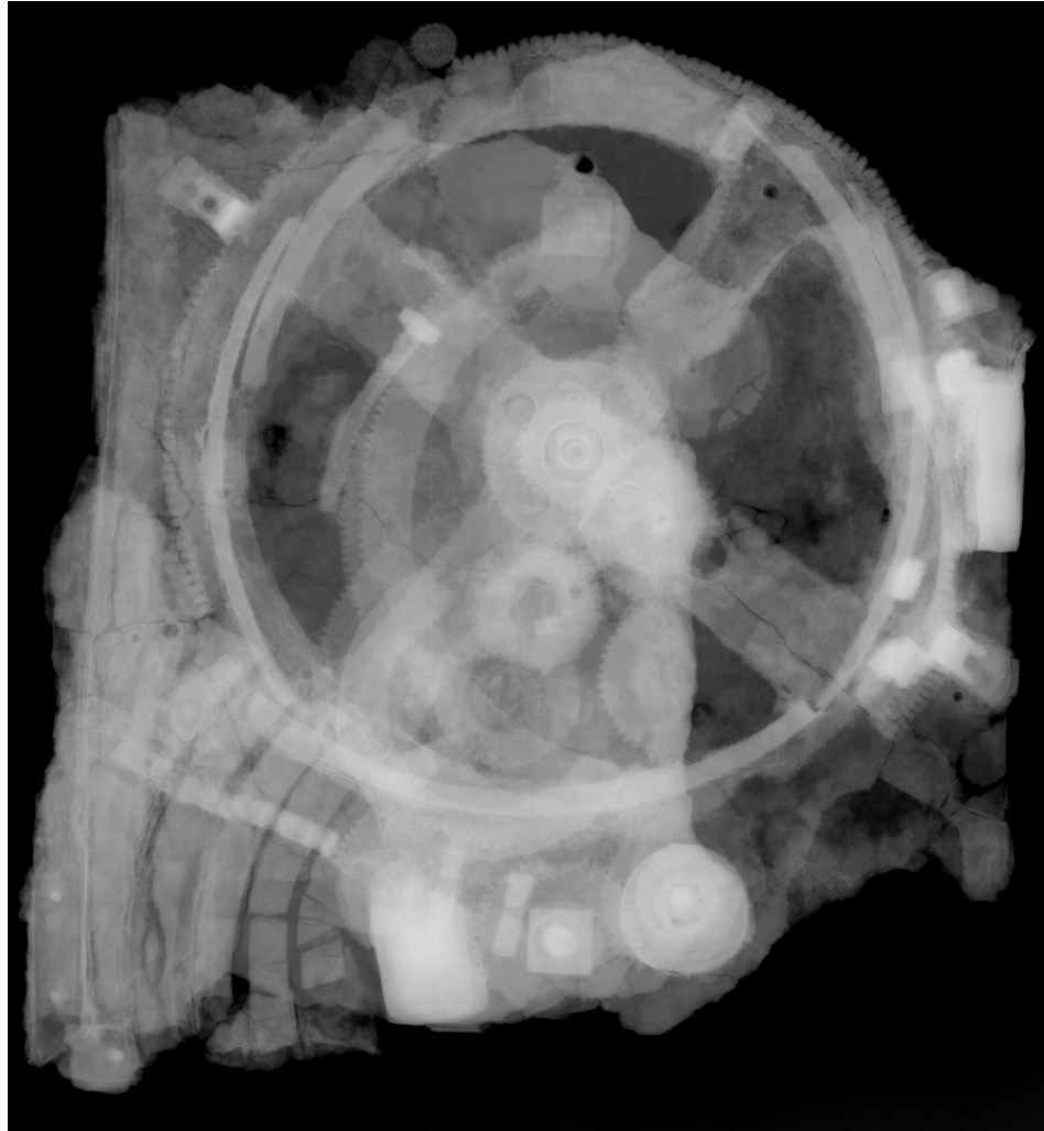
Figure 6.10: X-ray micro-focus computed tomography (CT) image of Fragment A. Clearly visible are all the inner gears, as well as many of the axes and irregular features. Even more than the outside of the fragment, this image illustrates the enormous complexity of the extraordinary Antikythera Mechanism.
