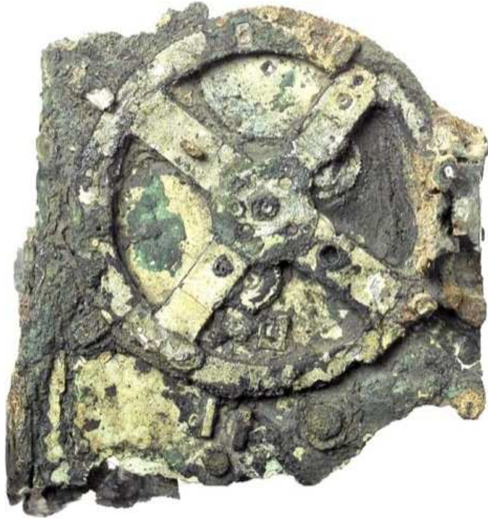
Figure 6.2: Front face of the largest surviving part; Fragment A. One of its main features is the large gear wheel on the front face, but it also directly manifests the complexity of the device; a vast diversity of gears, holes and pegs characterize the ancient complexity of this extraordinary mechanism immediately. The large gear wheel is now known as the Sun-wheel. It has 224 teeth, and figures as the main drive for the mechanical computer, in most reconstructions made by now.
