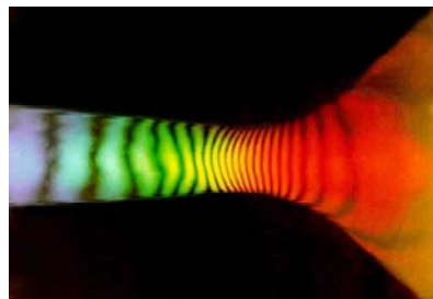
Two illustrations of the de Laval nozzle principle. The 2 nd figure is a measurement of the flow speed in an experiment.
