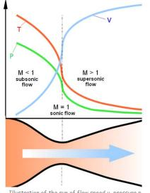
Illustration of the run of flow speed u, pressure p and temperature T, as the gas passes through the nozzle and its sonic point.
