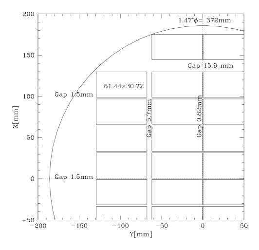
Figure 1. Lay out of the positioning of the CCD's in a quadrant of the OmegaCAM focal plane
