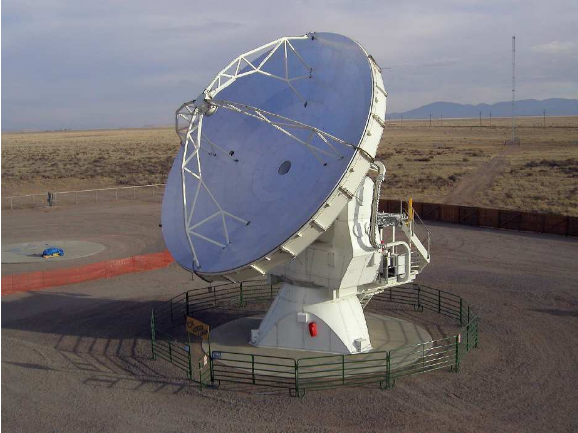
Figure 67: The ALMA VertexRSI prototype antennas is shown in PR Photo 06c/03 on the Antenna Test Facility (ATF) site at the NRAO Very Large Array (VLA) site near Socorro (New Mexico, USA).
