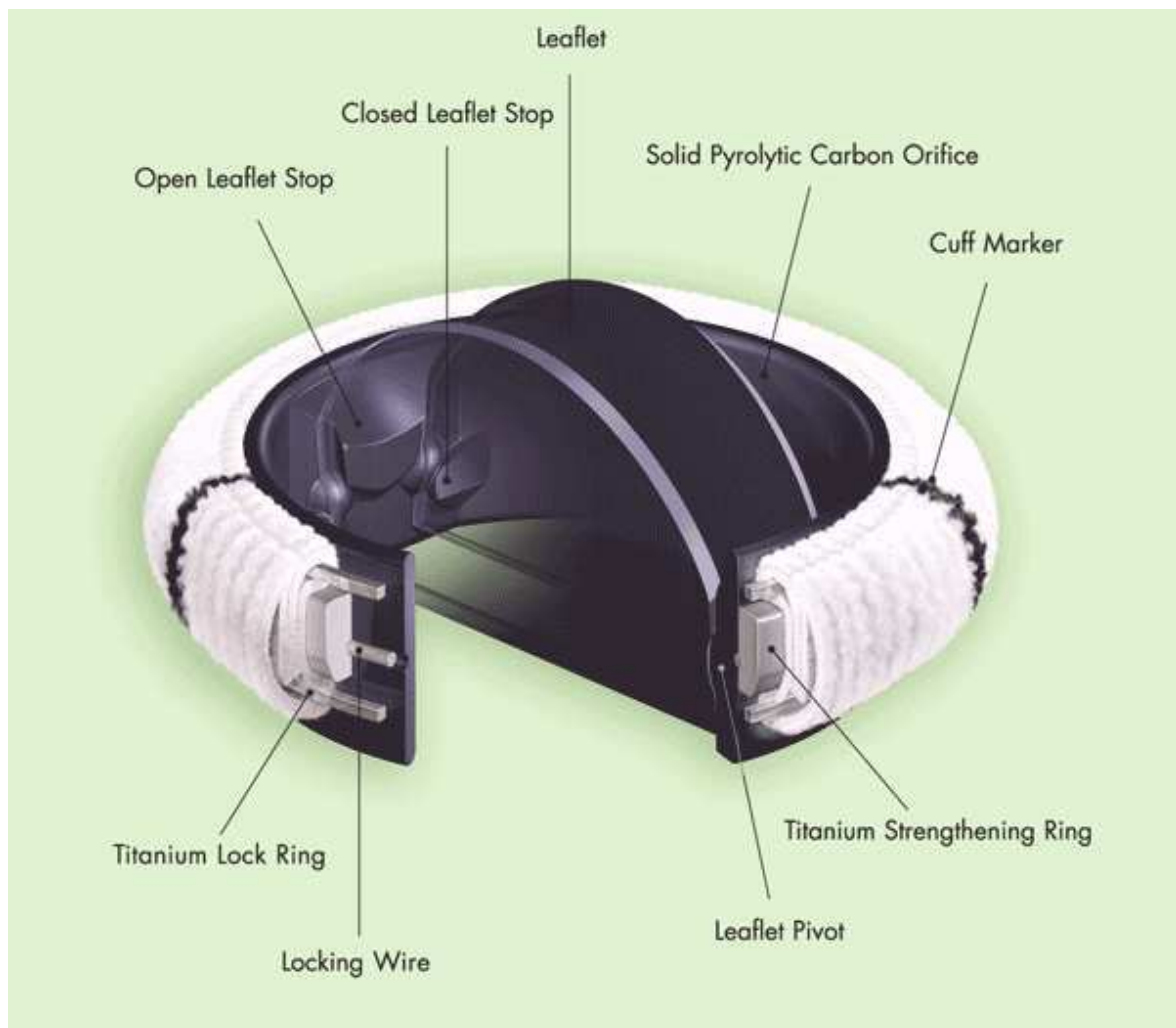
Figure 49: This shows a model of the artificial valve that was placed in my aorta during surgery. It is produced by ATS Medical, Minneapolis, U.S.A. The 'ATS Open Pivot Heart Valve' is composed of an orifice ring, two leaflets, and a polyester sewing cuff. The orifice ring is pure pyrolytic carbon for exceptional durability and maximal flow area. The leaflets incorporate a graphite substrate impregnated with 20% tungsten for enhanced radiopacity. The strengthening ring, lock rings, and lock-wire surrounding the pyrolytic carbon orifice are made of titanium for enhanced strength and radiopacity. It measures in my case 25 mm in diameter and should work for at least 30 years, which corresponds to 1 billion ( 10^9 ) times opening and closing.
