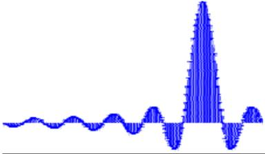
➔ Truncating the impulse response of an ideal filter to obtain a realizable filter, creates oscillatory behavior in the frequency domain.
