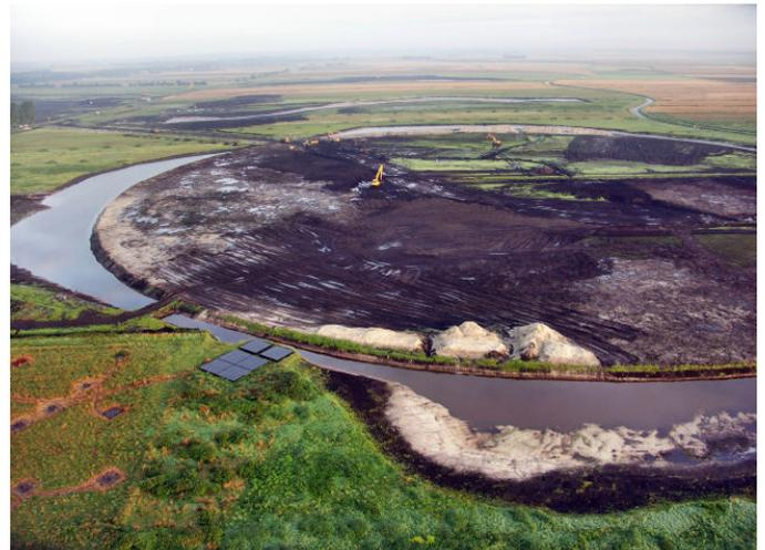
**Figure 6:** The central area of the LOFAR Core near the village of Exloo in the Netherlands. The inner circle has a diameter of 350 m, the total core area is approximately 2 km in diameter. In the lower left corner, part of a test station is visible. The black rectangles are High Band Antenna tiles. Some Low Band Antennas are only visible from the lack of vegetation around their groundplanes.
