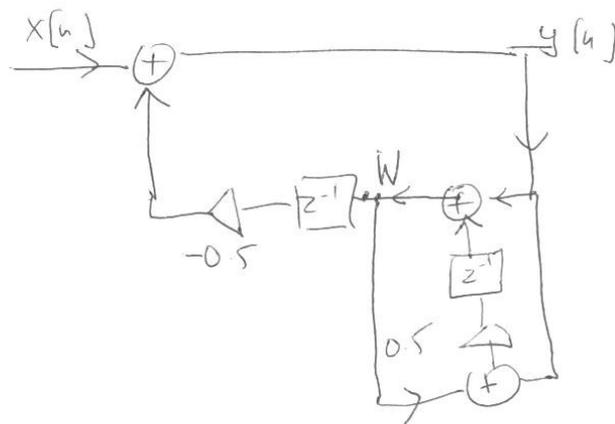
$$W[n] = y[n] + 0.5y[n-1] + 0.5W[n-1] \quad \text{or} \quad W = Y + 0.5z^{-1}Y + 0.5z^{-1}W$$
