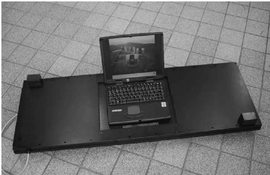
Figure 4. The OmegaCAM exposure shutter. The aperture size is 370 \times 292 mm, the shortest possible exposure time is smaller than 1msec, the deviations of the effective exposure time from pixel to pixel (homogeneity) are smaller than \pm 0.2\% for a 100msec exposure, the exposure time accuracy is about 0.3msec. The laptop is shown for scale.
