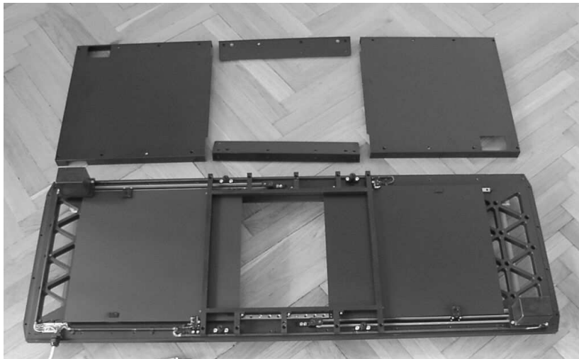
Figure 6: Picture of the partly disassembled shutter unit. The two blades, as well as the central aperture, are visible in the lower part of the unit.
