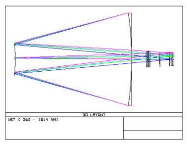
Fig. 1 - VST complete optical layout of telescope with one lens and the ADC, with a curve dewar window
